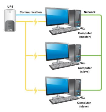
One UPS, multiple computers. Only one of them can actually talk to the UPS directly. That's where the network comes in. The Master system runs the driver, upsd, and upsmon in master mode. The Slave systems only run upsmon in slave mode.
